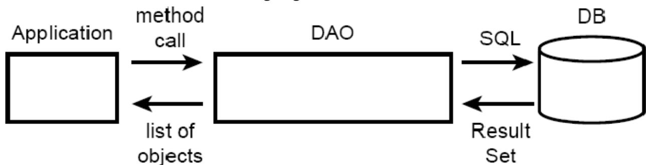
*Figure: Data Access Object design pattern*
